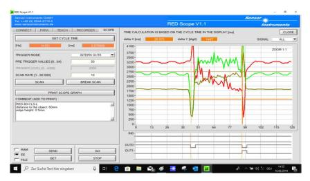
Signal evaluation of edge detector RED-60-CLS-L with the RED-Scope Windows® software.
